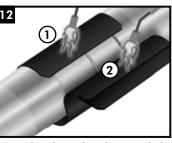
Wrap the sleeve loosely around the pipe, ensuring the appropriate overlap. Gently heat the backing of the underlap and the adhesive side of the overlap. Press the overlap into place.
