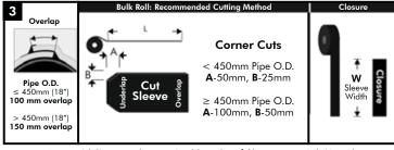
As a guideline, cut the required lengths of Sleeve material (L) and Closure material (W) from the bulk roll as follows L = Coated Pipe circumference + overlap dimension W = Sleeve Width
