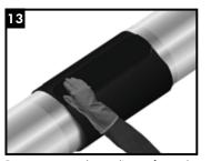
Remove any release liners from the Closure Strip. Centre the closure on the overlapping sleeve. Press down firmly.
