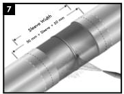
Ensure that the pipe is dry before cleaning. Prepare the steel joint area using the Surface Preparation and Pre-Heat Chart as a guideline. Lightly abrade the pipe coating adjacent to the cutback area to a distance of 50mm (2") beyond each end of the sleeve width.
