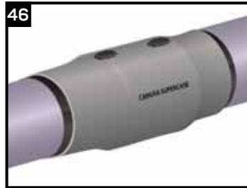
The CFS has been fully installed when adhesive can be seen around the entire circumference and is in full contact with the casing.
