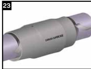
Carefully slide the CSC over the joint, so that the edges are centered over the edge of the adhesive strips.
