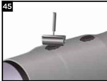
Using a roller, gloved hand or the side of the larger end of the CFS Rolling Tool; smooth out the CFS surface. Ensure adhesive has oozed from all sides of the CFS.
