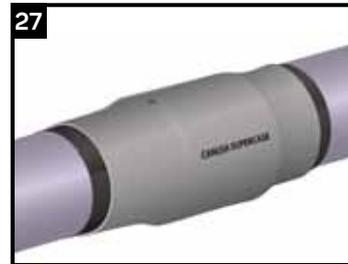
Continue heating the edge until it is fully recovered around the entire circumference of the jacket pipe. **Shrinking has been completed when the shrink zone of the CSC has conformed to the entire pipe jacket.**
