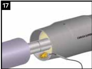
Pre-warm the inside of the casing on each end (150mm) by moving it half-way over the joint. Use low intensity flame to make sure that the casing does not start to recover.
