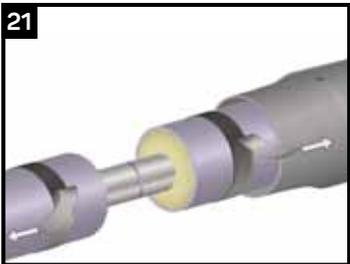
Fold the release liner outwards to allow for easy removal after positioning the casing.
