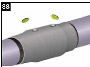
Continue with step 41 when the foaming hole is to be double sealed with a weldable plug and Canusa Foam Seal - CFS.
