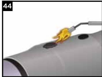
Using a weak medium flame, heat the backside of the CFS until the adhesive oozes from the edge and the thermo-chromic ink print disappears. Do not overheat the surface as the foam will gas.
