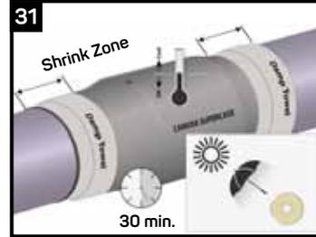
Allow the CSC to cool for 30 minutes. After 30 minutes measure the surface temperature of the CSC shrink zones. If the surface temperature of the shrink zones are still above 40°C, use shading and/or damp towels to quicken CSC shrink zone cooling time.
