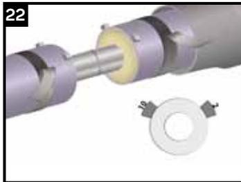
Remove the paper backing and place the spacers at the 10 and 2 o'clock positions of the jacket pipe, right at the edge of the cutback.
