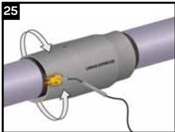
Using broad strokes and a medium flame, begin shrinking one end of the CSC evenly all around. Keep the torch moving to avoid overheating any spots; ensure sufficient heat is applied at the bottom.
