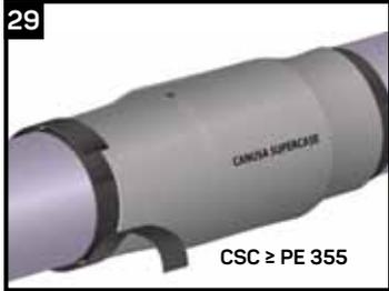
For casing sizes PE355 and above, wrap the supplied tension tape around the edge immediately after shrinking, while the casing is still soft (if the casing has cooled down; reheat it). This ensures even cooling and conformance of the edges.
