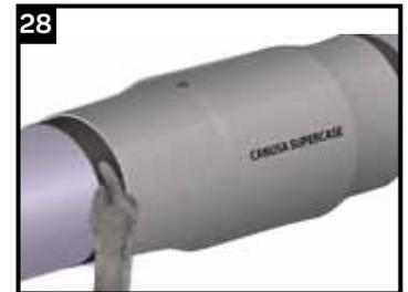
As a final check, ensure that the shrink zone of the CSC conforms intimately with the entire pipe surface. This can be checked by feeling the edges all around the circumference of the casing. If there is edge lifting, the edge should be reworked with additional heat.
