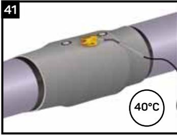
Pre-warm the casing surface around the foaming hole to 40°C. Do not overheat the surface as the foam will gas. Check the temperature using a temperature measuring device.
