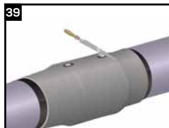
Using a grater, sand down the plugs bringing them flush to the surface of the CSC.
