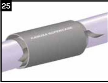
Carefully slide the CSC-X over the joint, so that the edges are centered over the edge of the adhesive strips.
