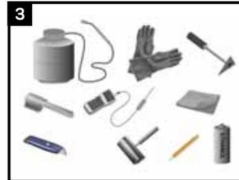
Propane tank, hose, torch & regulator; Sandpaper (40-60 grade) or wire brush; Knife, roller, rags & ethanol (min. 94%) cleanser; Temperature measuring device, Marking pencil; Standard safety equipment; gloves, goggles, hard hat, etc.
