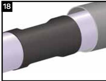
Tightly wrap the film around the pipe, ensuring the overlap is sufficient. Visually inspect the wrapped film for the following:
