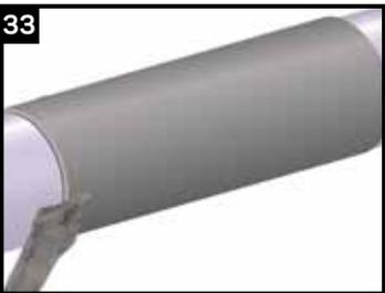
As a final check, ensure that the entire CSC-X conforms intimately with the entire pipe surface. This can be checked by feeling the edges all around the circumference of the casing. If there is edge lifting, the edge should be reworked with additional heat.
