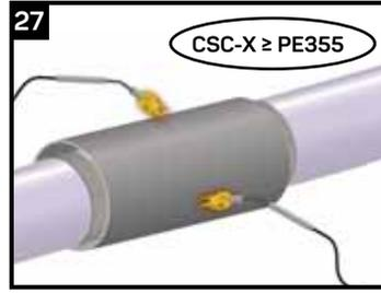
For CSC-X sizes 355mm and greater, it is recommended to use two installers working on opposite sides of the pipe. Using broad strokes and a medium flame, begin shrinking in the center of the CSC-X.
