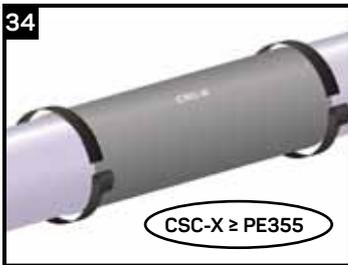
For casing sizes PE355 and above, wrap the supplied tension tape around both edges immediately after shrinking, while the casing is still soft (if the casing has cooled down; reheat it). **This ensures even cooling and conformance of the edges.**
