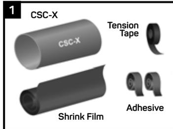
The fully shrinkable Canusa SuperCase™ - CSC-X is a crosslinked, heat shrinkable casing system for pre-foamed or foam half-shell filled joints on pre-insulated pipes. The CSC-X uses Shrink Film - WC-20R and SuperCase Adhesive - SA to seal the joints.
