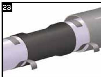
...apply the adhesive strips tightly around the jacket pipe with the mesh side facing up. The strips should be applied so that they are placed approximately 5mm inside of the marks. Make sure the adhesive is not stretched during wrapping. Partially peel-back the release liner on the under lap and wrap the strips around the jacket pipe so that they overlap.
