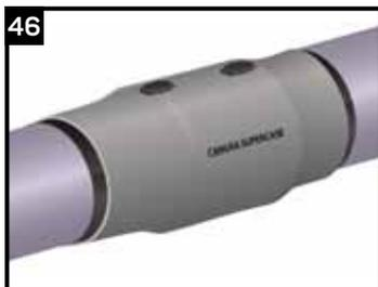
The CFS has been fully installed when adhesive can be seen around the entire circumference and is in full contact with the casing.
