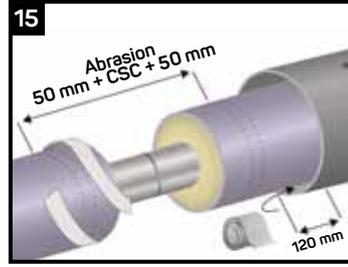
Roughen the surface of the jacket pipe on both sides of the cutback and the **inside of the CSC** using the sandpaper (40 to 60 grade).
