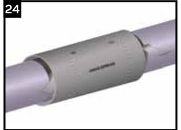
Carefully slide the CSC over the joint, so that the edges are centered over the edge of the adhesive strips.
