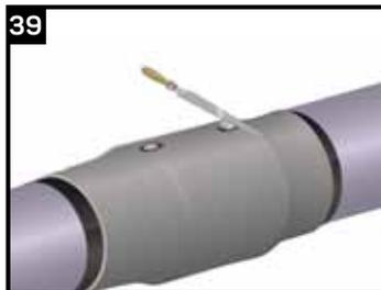
Using a grater, sand down the plugs bringing them flush to the surface of the CSC.
