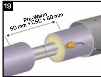
Pre-warm the pipe to 40°C-50°C. **Ensure the correct temperature with a temperature measuring device.** Do not exceed 60°C as this makes the removal of release liner difficult.
