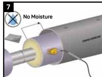
Use a propane torch with a **low flame** to dry the jacket pipe, carrier pipe and CSC. Use a dry, grease and lint-free rag to wipe clean the jacket pipe, carrier pipe and CSC.
