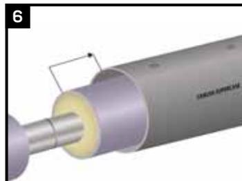
**Check the CSC to ensure that it is not damaged.** Before welding together the carrier pipes, slide the CSC as far away from the joint as possible.
