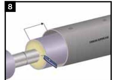
**Remove any wet PUR foam** from the end of the pre-insulated pipe.
