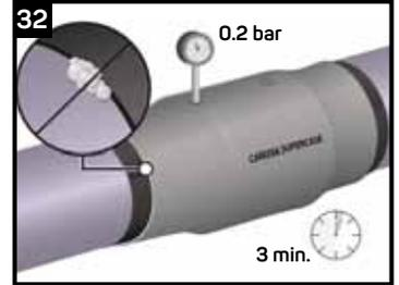
Ensure the CSC shrink zones have cooled to below 40°C. Perform the pressure test using the previously drilled pressure hole. The CSC should be checked with an air pressure test for 3 minutes at 0.2 bar. In case of a leak, the CSC shrink zones should be reworked with additional heat at the leaking area. The pressure test should then be repeated.
