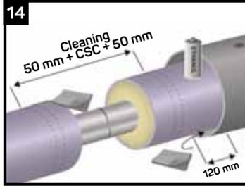
Clean the surface of the jacket pipe and the inside of the end zone of the casing with a rag to remove dirt. De-grease the surface of the jacket pipe and the inside of the CSC using a grease and lint-free rag soaked in ethanol (min. 94%) or isopropyl alcohol cleanser.
