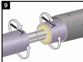
Using a triangular scraper, clean the edges of the jacket pipe to remove any burrs and dirt from the sealing area.
