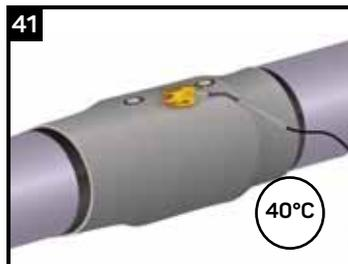
Pre-warm the casing surface around the foaming hole to 40°C. **Do not overheat the surface as the foam will gas.** Check the temperature using a temperature measuring device.
