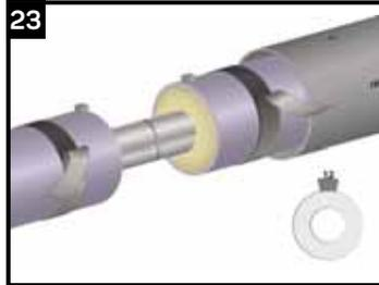
Remove the paper backing and place the spacer at the 12 o'clock position of the jacket pipe, right at the edge of the cutbacks. Note: The use of spacers is optional, but recommended.
