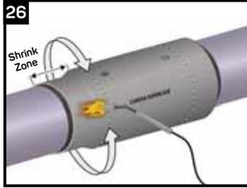
Using broad strokes and the appropriate flame, begin shrinking one end of the CSC evenly all around. Keep the torch moving to avoid overheating any spots; ensure sufficient heat is applied at the bottom. **Ensure the flame remains in the shrink zone and the torch is never pointed at the CSC middle or jacket pipe.**
