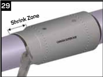
As a final check, ensure that the shrink zone of the CSC conforms intimately with the entire pipe surface. This can be checked by feeling the edges all around the circumference of the casing. If there is edge lifting, the edge should be reworked with additional heat.
