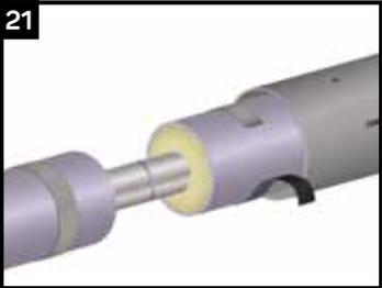
...apply the adhesive strips tightly around the jacket pipe with the mesh side facing up. The strips should be applied so that they are placed approximately 5mm inside of the marks. Make sure the adhesive is not stretched during wrapping. Partially peel-back the release liner on the under lap and wrap the strips around the jacket pipe so that they overlap.
