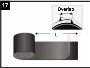
If not using the pre-cut adhesive from a kit, measure the circumference of the jacket pipe and cut two sealing strips long enough to allow for overlap.
