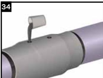
**The temperature of the CSC shrink zones should not be more than 40°C when foaming.** If necessary, follow the cooling instructions as described in step 32 to ensure the CSC shrink zones are below 40°C.
