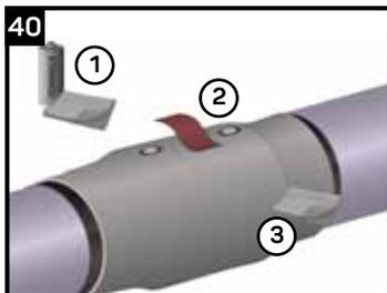
1. De-grease the surface around the plug using a grease and lint-free rag soaked in ethanol.
