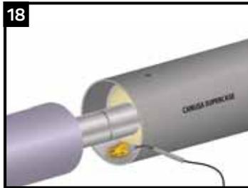
Pre-warm the inside of the casing on each end (150mm) by moving it half-way over the joint. Use low intensity flame to make sure that the casing does not start to recover.
