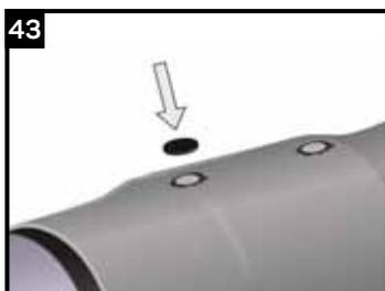
Place the CFS onto the pre-cleaned and pre-warmed section of casing directly over the centre of the foaming hole.
