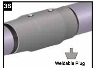
After the foam has hardened, remove the ventilation plugs and drill any holes necessary for sealing. When using Canusa approved weldable plugs and welding machine, it is required to match the conical geometry with all pieces of equipment (i.e. weldable plug, drill bit, welding machine heating cups). Cylindrical tools for plug welding are not recommended. Note: Using an approved welding tool, (at 250 the recommended times for plug welding are:
