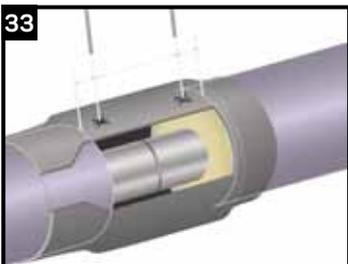
Drill one foaming hole over the pressure testing hole. Drill the other foaming hole, if required through the centre of the other foam hole welding puck.
