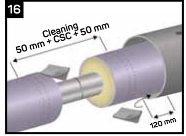
Using a dry, grease and lint-free rag, clean the roughened surface to remove any polyethylene or sand particles.
