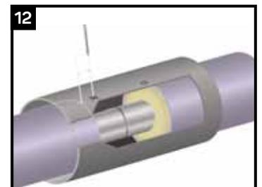
Drill a hole for air pressure relief through the centre of one of the foam hole welding pucks to allow air to escape during installation. **Ensure no damage is done to the jacket pipe.**
