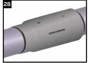
Continue heating the edge until it is fully recovered around the entire circumference of the jacket pipe. **Shrinking has been completed when the shrink zone of the CSC has conformed to the entire pipe jacket.**
