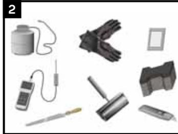
Propane tank, hose, regulator and torch; wet film thickness gauge; mixing sticks, cups and applicator pads; digital thermometer with suitable probe sleeve roller; appropriate tools for abrasion; standard safety equipment (gloves, goggles, hard hat, etc.)
