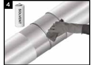
Ensure that the mainline coating edges are beveled to 30°. If there is the presence of oil, grease, or other surface contaminants; clean the exposed steel and adjacent pipe coating with a solvent cleanser.
