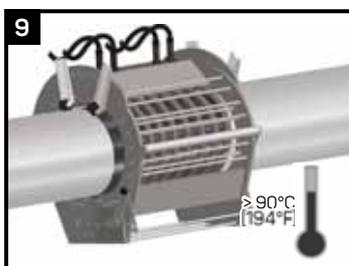
Using the appropriate sized induction coil or propane torch(es), pre-heat the joint area to > 90°C (194°F). When heating with torch, use heat shields to protect mainline coating from the flame. Using a temperature measuring device, ensure that the correct temperature is reached on the steel and the coating overlap which the sleeve will cover. Check to ensure the correct minimum temperature has been achieved on each quadrant of the bare steel cutback surface and mainline coating overlaps.
