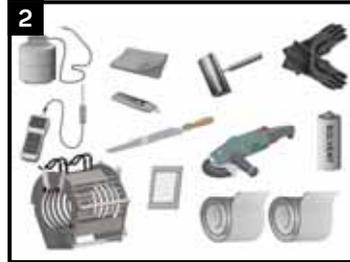
Propane tank, hose, torch & regulator; Power grinder with grind wheel of a Grade 40 grit rating; Canusa heat shields; Induction coil & generator; Digital thermometer with suitable probe; Knife, J roller, rags & approved solvent cleanser; Epoxy applicator pad, wet film thickness gauge; Standard safety equipment; gloves, goggles, hard hat, etc.
