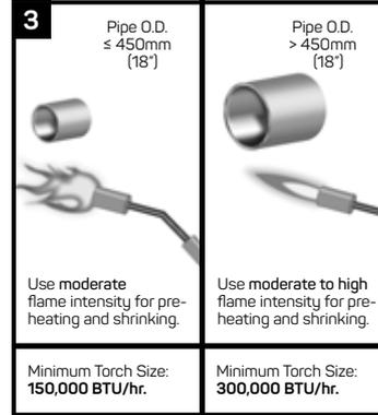
Use moderate flame intensity for pre-heating and shrinking.
