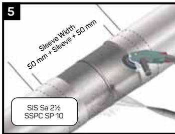
Warm the joint area to 40-50°C (100-120°F) before grit blasting. Thoroughly clean the weld area with a sand or grit blaster to "near white metal" SIS Sa 2½ or equivalent. Abrade the mainline coating adjacent to the weld area to a distance 50 mm (2") beyond the sleeve width.
