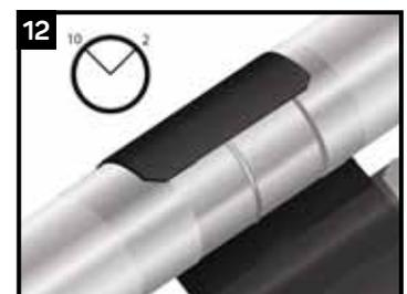
Place the underlap of the sleeve onto the joint, centering the sleeve such that the sleeve overlap is positioned at either the 10 or 2 o'clock position. Ensure that the sleeve is placed square to the pipe.
