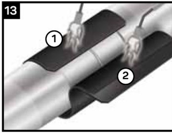
Remove the remaining sleeve release liner and wrap the sleeve loosely around the pipe, ensuring the appropriate overlap. Before finishing wrapping the sleeve:
