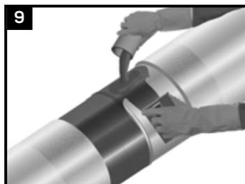
Apply mixed epoxy to a thickness of 150-230 µm (6-9 mils) on all exposed bare metal.
