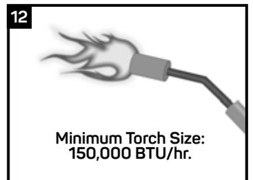
Use moderate flame intensity for sleeve shrinking. Remove protective heat shields prior to next step.
