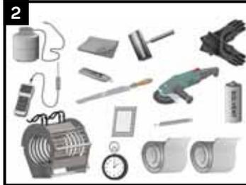
Propane tank, hose, torch & regulator; Appropriately sized induction coil, stop watch; Tools for surface abrasion, power grinder; Digital thermometer with suitable probe; Spacer Blocks (recommended); Protective Heat Shields (pre-sized for the pipe diameter); Knife, pencil, roller, rags & approved solvent cleanser; Epoxy applicator pad, wet film thickness gauge; Standard safety equipment; gloves, goggles, hard hat, etc.
