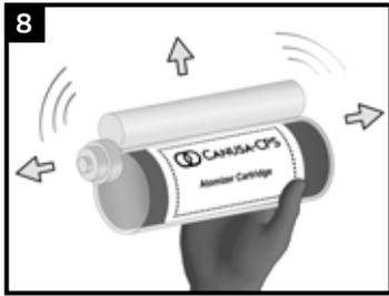
Once heated, the viscosity of the cure side will be very low. Holding the base side of the cartridge, shake the cartridge up and down and side to side to lightly redistribute the pigment colour in the cure side of the cartridge.
