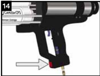
Press the red button to retreat fluid ejector pistons. Remove atomizing air hose from mixing tip and remove cartridge.
