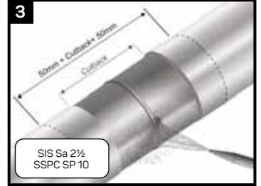
Thoroughly clean the cutback area to "near white metal" SIS Sa 2½ (SSPC-SP10) or equivalent. Materials used for abrasive blasting shall produce an angular surface profile of 2.5-5 mils (64-127 µm) Lightly abrade at least 50mm (2") of the line coating on each side of cutback area.
