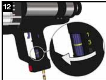
Adjust the atomizing air pressure dial to #3 +/- 1. This setting may vary depending on the temperature of the product and input air pressure.
