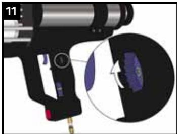
Adjust the fluid control dial to a setting of #3 +/- 1 by scrolling up or down. The dial is located on the side of the gun handle, behind the trigger. This setting regulates the speed/pressure of the two pistons. This setting may vary depending on temperature of product and input air supply pressure.
