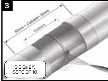
Thoroughly clean the cutback area to "near white metal" SIS Sa 2 1/2 (SSPC-SP10) or equivalent. Materials used for abrasive blasting shall produce an angular surface profile of 2.5-5 mils (64-127 µm). Lightly abrade at least 50mm (2") of the line coating on each side of cutback area.
