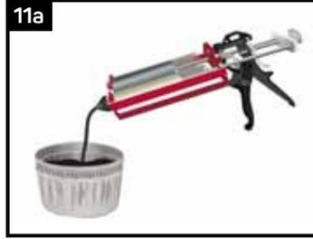
To dispense, unscrew the cap, remove the two small plugs in each side of the cartridge and replace cap. Squeeze the trigger of the cartridge dispenser and dispense a desired amount of material into a mixing cup. The cartridge dispenser will automatically dispense the correct ratio of base and cure.
