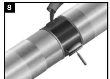
Dispense epoxy across the steel cutback and spread around the circumference of the pipe.
