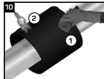
1. Clean the overlap area of the sleeve where the closure is to be applied.
