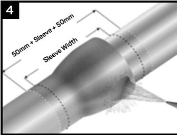
Ensure that the pipe is dry before cleaning. Prepare the steel joint area to a minimum of St2 /SP2. Lightly abrade the pipe coating adjacent to the weld area to a distance of 50mm (2") beyond each end of the sleeve width.
