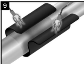
Wrap the WLOX sleeve around the tyton joint. Gently heat the backing of the underlap and the adhesive side of the overlap. Finish wrapping the sleeve around the tyton joint pressing the overlap firmly into place.
