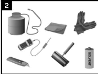
Propane tank & torch; Appropriate tools for surface abrasion; Knife, roller, rags & solvent cleanser; Temperature measuring device; Standard safety equipment; gloves, goggles, hard hat, etc.
