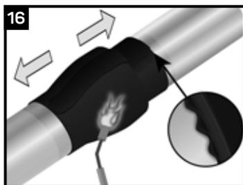
In a similar manner, heat and shrink the remaining side. Shrinking has been completed when the adhesive begins to ooze at the sleeve edges all around the circumference.
