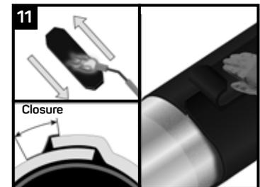
Warm the adhesive side of the closure until it becomes shiny. Centre the closure over the overlap. Using a gloved hand press the closure firmly down onto the overlapping sleeve.
