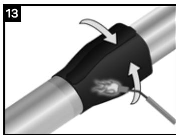
Using broad strokes, begin shrinking the sleeve around the entire circumference of the larger end (bell) of the tyton joint. Continue heating from the centre of the sleeve until sleeve recovery is completed around the bell of the tyton joint.
