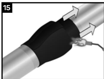
If the closure lifts while shrinking, secure it with a gloved hand. Continue heating from the bell of the tyton joint to the other end (spigot) until recovery is complete.
