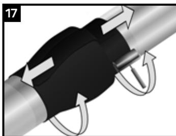
While the sleeve is still hot and soft, use a hand roller to firmly roll the sleeve surface and push any trapped air up and out of the sleeve, as shown above. If necessary, reheat to roll out air.
