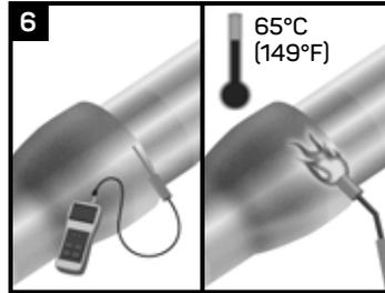
Pre-heat the joint area to a minimum of 65°C (149°F). Using a temperature measuring device, ensure that the correct temperature is reached on the steel and at least 50mm (2") on each side of the sleeve.
