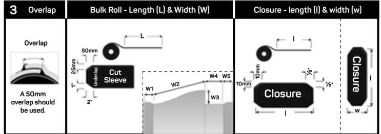
Cut the required length (L) of sleeve material from the bulk roll. The length should be calculated using the circumference of the joint + 150mm
