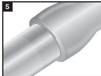
If a temporary seal is required, wrap the sealant rod around the pipe and press well into the bell face to fully cover the cavity.
