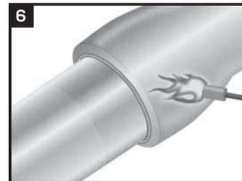
Pre-heat the joint to 50°C (120°F) using an appropriate heating device. (warm to the touch)
