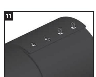
Insert the clips through the holes, push down the closure area to conform to the joint profile. Insert the flat-head screwdriver into the clips and then flatten the clips with gentle blows from a hammer (use needle-nose pliers if clips become bent or irregularly shaped).
