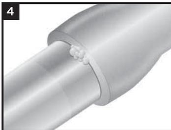
Check for leaks using soapy solution. Knock the lead in using a caulking tool to stop the leak. If necessary, use a non-melting caulking compound (e.g. Polychrestic Putty) to stop the leak. The joint must be dried before using any caulking compound.
