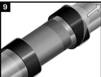
Remove the plastic bag from the tubular sleeve. Ensure that there is no dirt or moisture inside the tube and that the tube is not cut. If the sleeve is not useable, a one-piece Superseal pre-welded sleeve or Superseal bulk wrap sleeve should be used.
