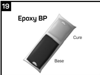
Follow the Preparation, Mixing and Application instructions provided with the supplied Canusa Epoxy Pack. For bulk quantities: mix the epoxy cure with the epoxy base (4 parts base to 1 part cure **by volume**). Stir for a minimum of 30 seconds to assure uniform mixture.
