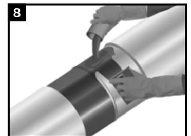
Apply mixed epoxy to a uniform specified thickness of 4-6 mils (100 - 150 microns) on all exposed bare metal using the applicator pads as supplied or an approved tool. Do not apply the epoxy to the mainline coating.
