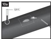
Using the propane torch, heat the repair area to 125°C. Using a digital thermometer, ensure the correct temperature has been reached.
