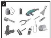
Propane tank, hose, torch & regulator; Appropriate tools for surface abrasion: grinder, 80-120 grit sandpaper; Appropriate tools for cleaning: rags & approved cleaner; Tools: roller, digital thermometer, knife, marker, measuring tape, scraper / spatula & pliers; Standard safety equipment; gloves, goggles, hard hat, etc.
