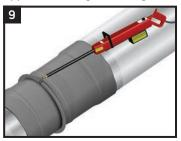
Joints covered with Syntho Poxy HC can be tested for pin holes and defects by the holiday method as per ASTM G62:
