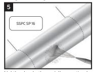
Lightly abrade the mainline coating by sweep blasting (preferred) to create a mechanical key without damaging the coating. SSPC-SP16 can be followed for this process.
