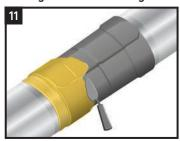
Apply Thermo-Poxy around the entire circumference of the pipe at a thickness of 100 microns. The epoxy will seal the surface of the treated pipe area and provide a great bonding to the composite system on the substrate.
