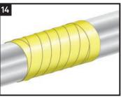
End wrap shall be vertical over itself (100%) unless further wrapping will proceed the next day or on joints; in this event the end wrap should remain in the wrapping direction.
