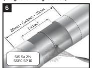
On joint weld areas, use Grit Blasting to reach a surface profile of SA2.5, SSPC-SP10, and remove excess rust, dirt or loose scale.
