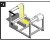
Pour Thermo-Poxy into the tray. Place the Thermo-Wrap 24 HDD roll on the input end of the Resinator machine and connect it through the resin box to the other end. Place the Thermo-Wrap 24 HDD roll on the input end of the Resinator machine and connect it through the resin box to the other end. Start rolling the handle of the Resinator to impregnate the roll.
