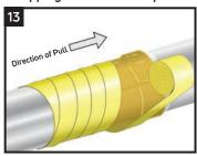
Application shall proceed while epoxy primer is wet/tacky. 2 layers of Thermo-Wrap 24 HDD is required and shall be applied in one run clockwise direction from right to left (R-T-L) or left to right (L-T-R) in a spiral manner around the pipe using a 50 % horizontal overlap. At the end of the first roll, attach the new roll lead at 200mm over the end roll and continue wrapping in the same manner.
