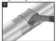
Acetone or other suitable solvent shall be used to wipe out the mainline coating and the blasted bare steel just before applying Syntho-Poxy. In case of heavy winds carrying dust and sand, the pipe shall be tented at the working area. Mobile tent is possible. The quality of the FBE coating or the mainline coating shall be checked before commencing composite wrap application.
