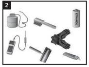
Canusa torch, propane tank, hose & regulator; Temperature measuring device, roller, knife; Appropriate surface abrasion device, solvent; Standard safety equipment (gloves, goggles, hard hat, etc.)
