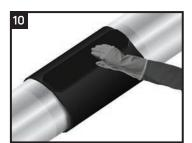
Press the closure firmly into place. Gently heat the closure and pat it down with a gloved hand. Repeating this procedure, move from one side to the other. Smooth any wrinkles by gently working them outward from the centre of the closure with a roller
