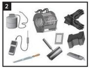
Propane tank, hose, torch & regulator; Appropriate tools for surface abrasion; Epoxy application accessories & wet film thickness gauge; Knife, roller, rags & Canusa approved solvent cleanser; Digital thermometer with suitable probe; Standard safety equipment: gloves, gogqles, hard hat, etc.
