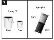
Follow the Preparation, Mixing and Application instructions provided with the supplied Canusa Epoxy Type S-80. For bulk quantities: mix the primer cure with the primer base (4 parts base to 1 part cure by volume). Stir for a minimum of 1 minute to assure uniform mixture.
