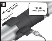
sleeve and 100 mm (4") onto the coating is at the required temperature. Completely remove any release liners from the sacrificial sleeve if present. Wrap the sacrificial sleeve so that half of the sleeve overlaps the primary sleeve and half of the sleeve extends onto the coating. Recover the sleeve as in steps 10 through 17, but position the closure on the opposite side of the pipe relative to the primary sleeve closure.
