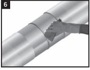
Using a dry, grease and lint-free cloth, wipe clean or air blast the steel and coated areas to remove foreign materials. If necessary, provide additional heat to ensure the surface temperature is 40-50°C (104-120°F).
