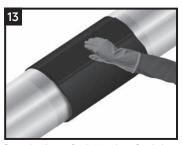
Press the closure firmly into place. Gently heat the closure and pat it down with a gloved hand. Repeating this procedure, move from one side to the other. Smooth any wrinkles by gently working them outward from the centre of the closure with a roller.
