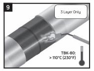
Pre-heat the joint area and abraded coating to the required temperature with the appropriate propane torch. If epoxy is applied, ensure that the epoxy is dry to the touch prior to sleeve installation. Do not use an intense flame on the mainline coating. If a film develops on the mainline coating because of preheat, use a surface abrasion tool to remove it.
