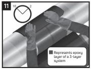
Centre the sleeve over the joint so that the sleeve overlaps between the 10 and 2 o'clock positions. Press the underlap firmly into place. Remove the remaining release liner.
