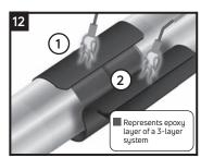
Wrap the sleeve loosely around the pipe, ensuring the appropriate overlap. Gently heat the backing of the underlap (1) and the adhesive side of the closure until it becomes shinu.
