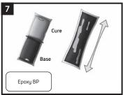
Follow the Preparation, Mixing and Application instructions provided with the supplied Canusa Epoxy Pack. For bulk quantities: mix the epoxy cure with the epoxy base (4 parts base to 1 part cure by volume). Stir for a minimum of 30 seconds to assure uniform mixture.
