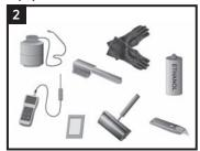
Canusa torch, propane tank, hose & regulator; Temperature measuring device, roller, knife; Appropriate surface abrasion device, solvent; Standard safety equipment (gloves, goggles, hard hat, etc.); Wet film thickness gauge
