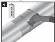
Ensure that the mainline coating edges are bevelled to 30°. If there is the presence of oil, grease, or other surface contaminants; clean the exposed steel and adjacent pipe coating with a solvent cleanser.
