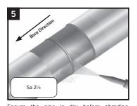
Ensure the pipe is dry before abrading. Thoroughly clean the weld area with a sand or grit blaster to "near white metal" SIS Sa 2% or equivalent. Lightly abrade the mainline coating adjacent to the cutback edge to a distance that is at least 25 mm beyond the edge of all joint coating, which includes the primary and sacrificial sleeves.
