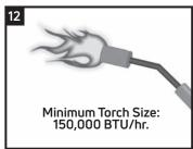
Use moderate flame intensity for sleeve shrinking. Remove protective heat shields prior to next step.
