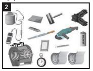
Propane tank, hose, torch & regulator; Appropriately sized induction coil, stop watch; Tools for surface abrasion, power grinder; Digital thermometer with suitable probe; Spacer Blocks (recommended); Protective Heat Shields (presized for the pipe diameter); Knife, pencil, roller, rags & approved solvent cleanser; Epoxy applicator pad, wet film thickness gauge; Standard safety equipment; gloves, goggles, hard hat, etc.
