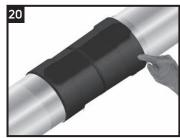
Test sleeve adhesion by gently pulling the edge of the backing back to ensure that the adhesive remains in place and is fully bonded to the factory coating. The sleeve is well bonded when the adhesive and coating remain intimately contacted. If required to improve bonding, additional heat should be applied to the sleeve. Remove protective heat shields when application is completed.
