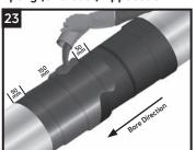
When the sleeve is between 15 - 40°C, apply epoxy over the sacrificial sleeve to form a wear cone; covering 50mm (2") onto the pipe coating, the entire sacrificial sleeve and 50mm (2") onto the first sleeve. Epoxy applied should thoroughly cover the edge of the sleeves.
