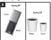
Follow the preparation, mixing and applications instructions provided with the supplied Canusa Liquid Epoxy Pack. For bulk quantities, mix the epoxy cure with epoxy base (see Liquid Epoxy Product data sheet for mixing ratio). Stir for a minimum of 1 minute to assure uniform mixture.
