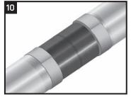
Heat shields are to be wrapped tightly around the overlap edges to prevent the mainline coating from potentially lifting during pre-heating. Ensure that the heat shields are not in contact with the epoxy coated cutback area.
