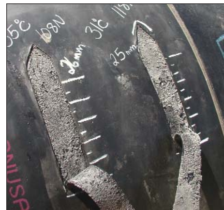
Figure 2. 3-layer coating and 3-layer sleeve compatibility.
