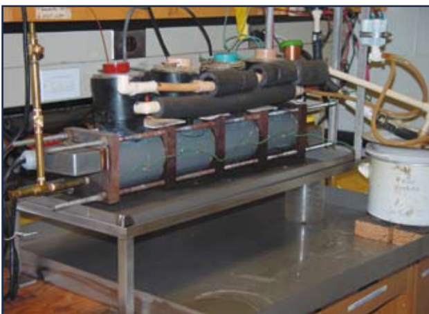
Figure 3. High temperature CD apparatus. Photo courtesy of ShawCor Ltd.
