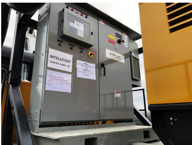
Figure 3. IntelliCOAT Control Panel equipped with PLC and touch-screen interface.
